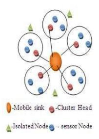
During data transmission the isolated nodes are allowed to transmit their sensed data either to the nearby CH or to the mobile sink. It is based on the shortest distance to the isolated node. The residual energy is also taken into consideration for data transmission.
